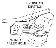
Figure 5. Engine Oil Dipstick
